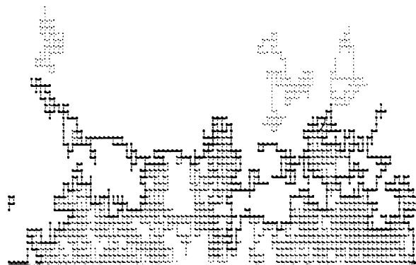
Figure 18. Polymer-polymer interface (one side) simulation on a 2D lattice. The interface was formed by reptation of random-coil interpenetrated chains of length 100 steps.
